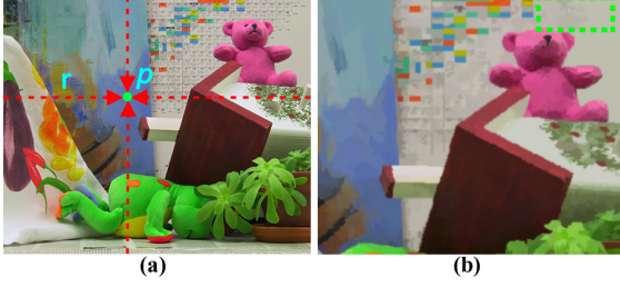
Fig. 1: (a) Path directions used for scanline optimization and (b) the (zoomed in) mean-shift segmentation map of the left “Teddy” image.
