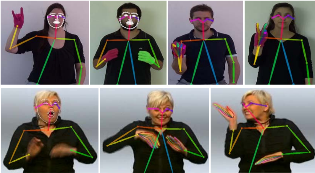
Figure 3: Examples of body/hand and body/face extraction from LSA64 (first row) and RWTH-PHOENIX (second row) datasets as the computational complexity of detecting all three skeletal features simultaneously was too heavy for our setup.
