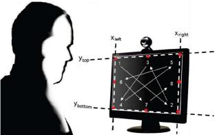
Fig. 4 Gaze-tracking framework setup and calibration procedure.
