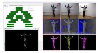
Fig. 2. Skeletal fusion from three Kinect sensors
