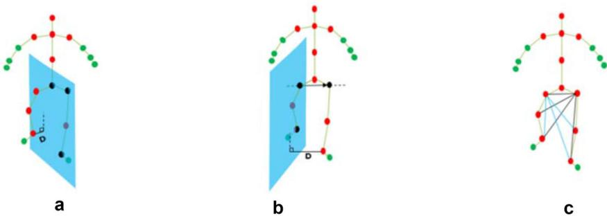
**Fig. 5** **a**  $D$  distance between right ankle and the plane defined by (pelvis, left hip, left ankle). **b**  $D$  distance between left ankle and the plane fixed in right ankle and normal to vector right hip  $\rightarrow$  left hip. **c** Example of relative motion
