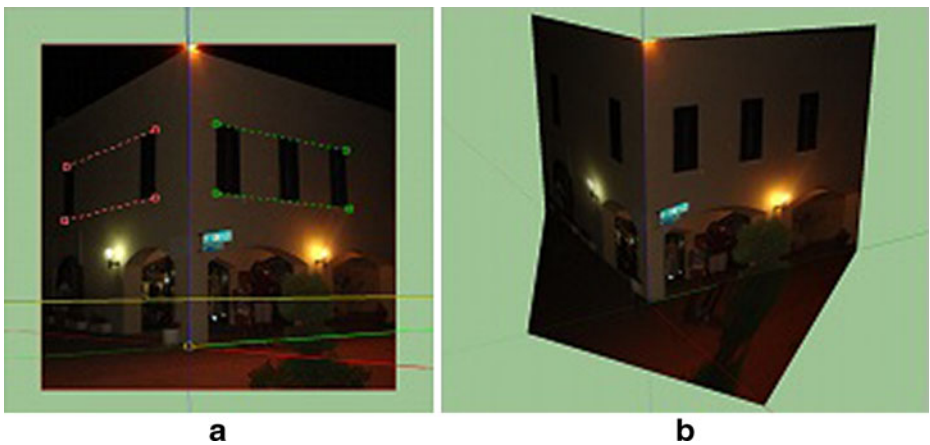
Fig. 13 a Presentation of Google Sketch-Up. b The produced 3D model
