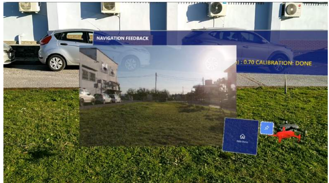
Figure 2. First Person View (FPV) into the Augmented Reality environment. Real and virtual drones are shown in the lower right corner.
