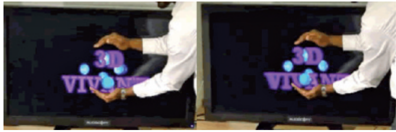
Figure 5. Two perspective views of a 3D holoscopic image on a commercial 3D autostereoscopic display. Parts of the 3D holoscopic image on the screen (such as the first globe) are visible at the same depth as the real hand.
