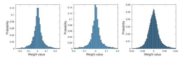
Figure 3: Weight values of linear convolution filter weights (left), Volterra-based convolution first-order weights (middle) and Volterra-based convolution second-order weights (right).
