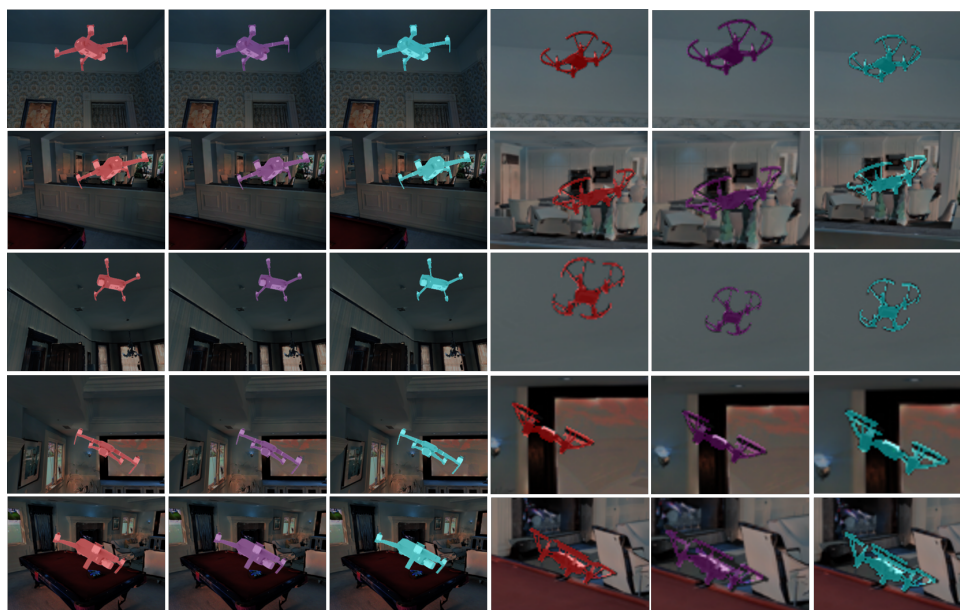
Figure 3. Qualitative results on random samples from the UAVA dataset from three different models. The red mask indicates predictions by l_p trained model, purple by l_m and finally cyan by HRNet. The drone masks are rendered by employing the predicted pose (i.e. output of the BPnP) and then blended with the original color image. The first three columns depicts M2ED drone model while the rest three the Tello drone. The Tello samples are cropped and zoomed-in due to its small form factor.
