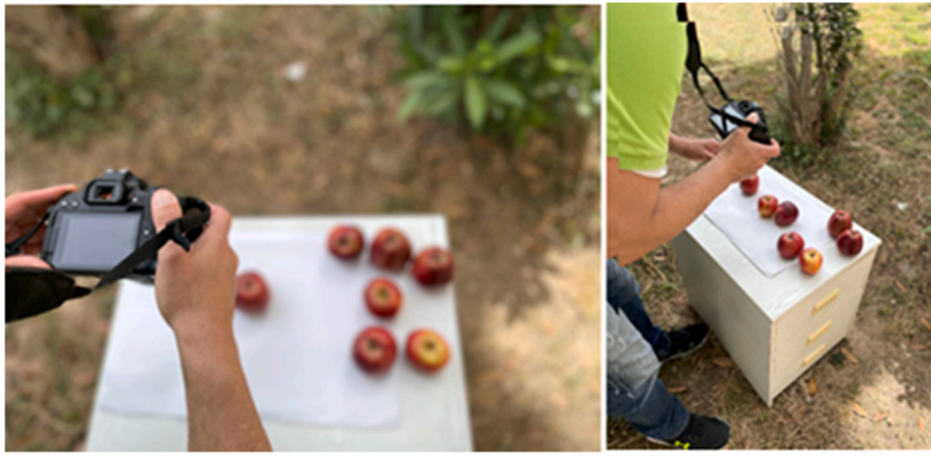
Fig. 4. Experimental setup for obtaining RGB images of apples using a white background and constant camera height of 20 cm above the samples.
