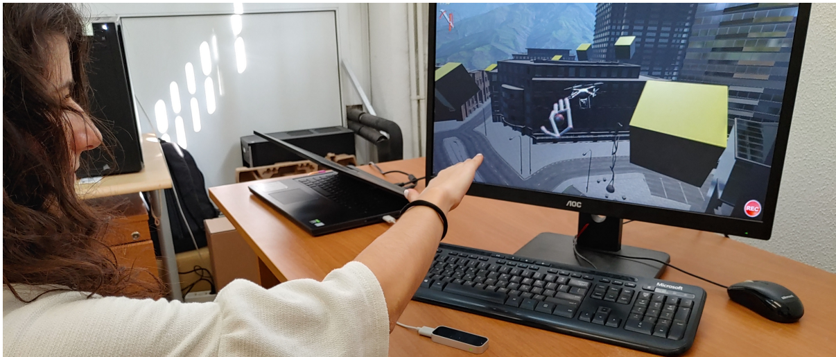
Figure 7. A user trying the palm-based controls. The open palm, held above the LeapMotion sensor is tilted to the left, corresponding to a left roll for the virtual UAV.
