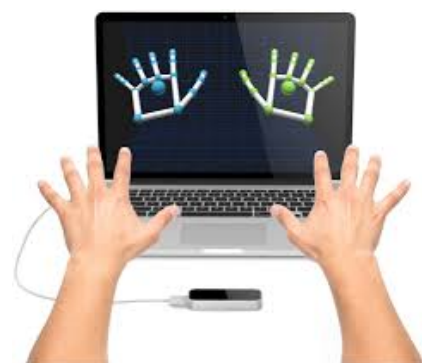
Figure 3. A LeapMotion sensor connected to a laptop showing the virtual hands.
