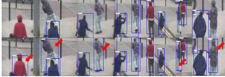
Fig. 7. Example detections on a MET CCTV video by the default PVANet.
