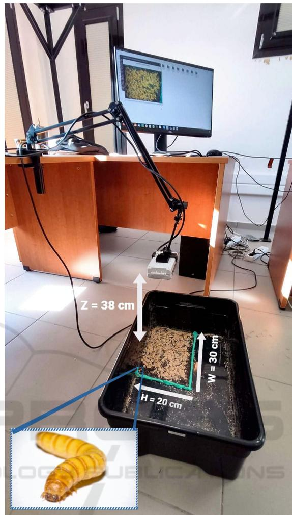
Figure 2: Experimental setup. The UI camera is placed at a 38 cm distance from the black crate, according to Equation 1. The spatial field of view is 20 x 30 cm. The camera is steadily placed on the desk during the whole experimental procedure.
