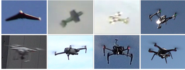
FIGURE 2. Examples of drone types present in the training set, i.e., Parrot Disco, 2 custom fixed-wing drones, DJI Inspire, DJI Phantom, DJI Mavic, DJI Matrice and 3DR Solo Robotics.
