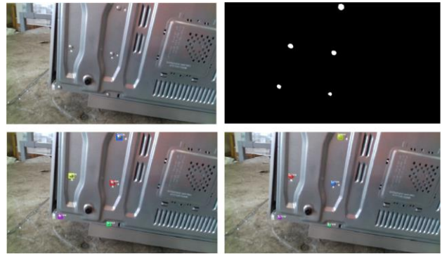
Fig. 3. Screw annotations for Semantic Segmentation, Object Detection and Instance Segmentation respectively.
