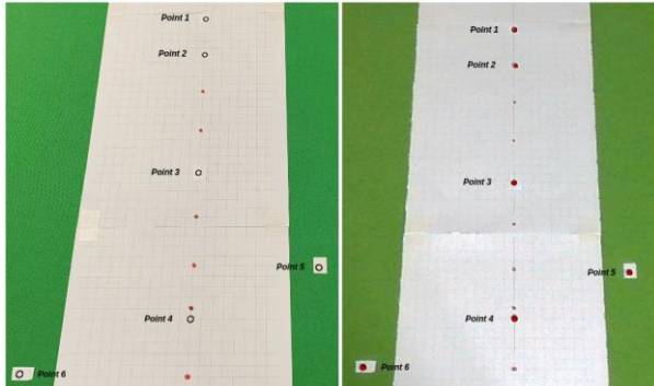
Fig. 4. Left: 2D Printed screws. Right: PointStamped messages after Deprojection in 3D space.
