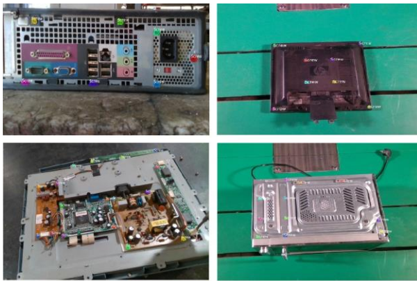
Fig. 2. Screw examples for different WEEE devices.
