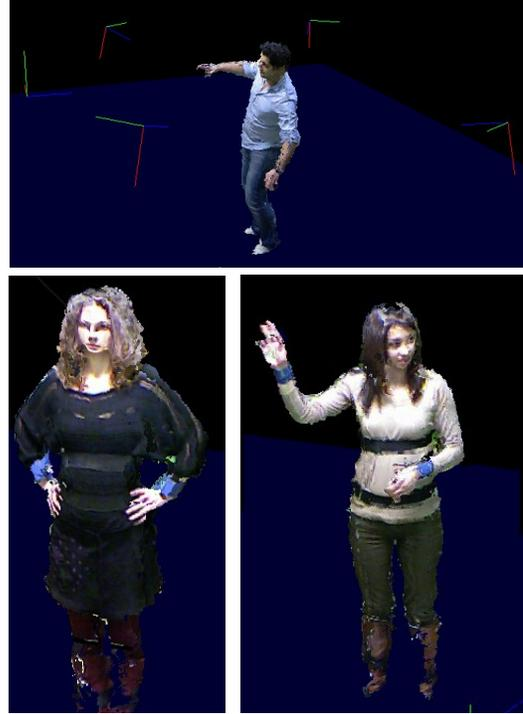
**Figure 4 Examples of real-time reconstructions. In the upper row, the colored lines indicate the positions and orientations of the cameras.**
